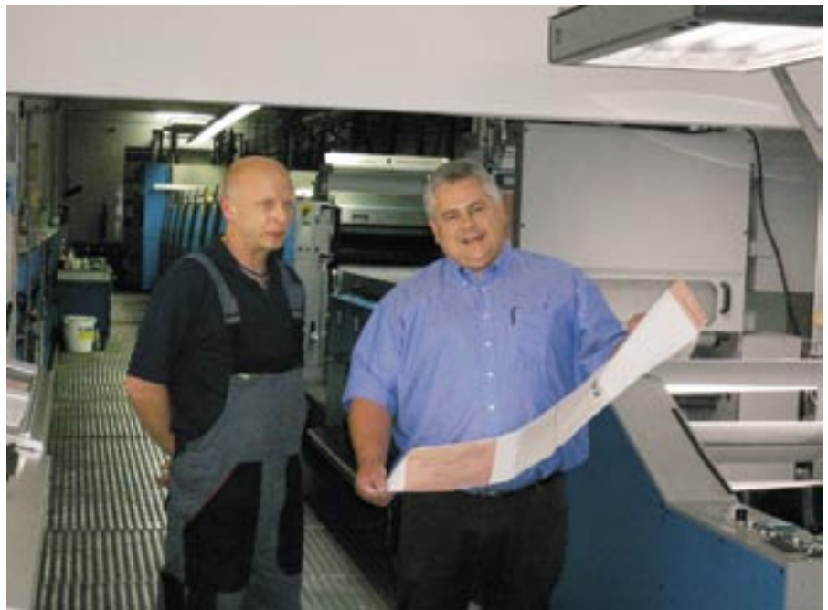
Managing Director Detlef Horn (right) and printer Uwe Choinowski next to an Alprinta 74 from Müller Martini (10 printing units in 32" and 40" format with a printing width of 740 mm).
